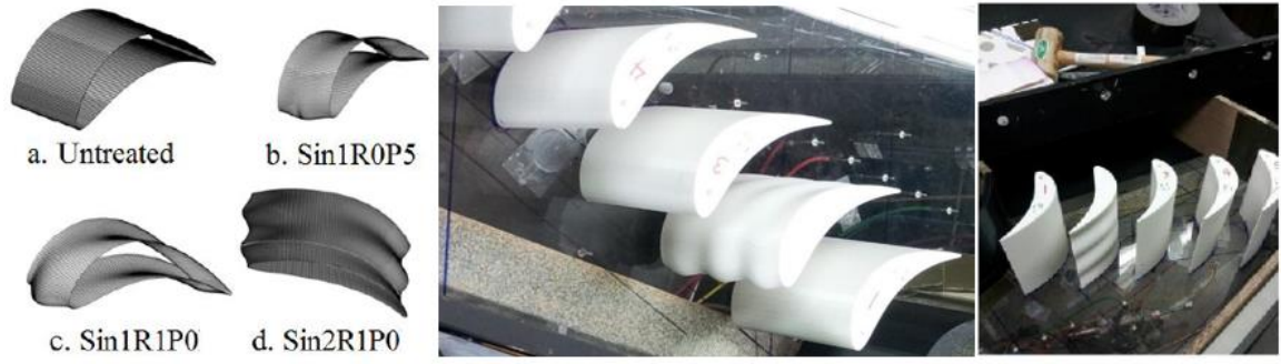
Figure 2.25 Harbor seal whisker inspired turbine blade geometries (Shyam et al., 2015)
