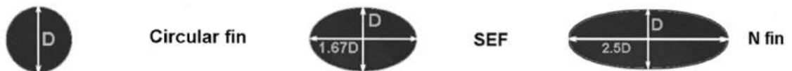
Figure 2.12 Pin model: Circular pin, Standard elliptical pin (SEF) and pin based on NACA 0024 (N fin) (Uzol & Camci, 2005)
