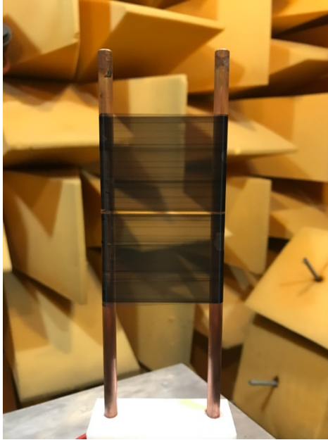
Figure 4-3: Picture of the CNT speaker used in this study. Note the CNT was not wrapped on both sides of the copper rods (i.e. it was single sided).
