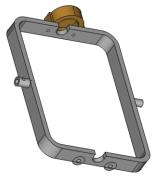
Figure 2.4: 3-D printed major platform showing pivots and casing for stepper motor
