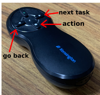
Figure 28: This example clicker has three buttons - the “next task” button goes to the next phase in the experiment, the “go back” button returns to the previous phase in the experiment, and the “action” button does an action, such as take a position measurement or blank or unblank the screen, depending on the trial phase.
