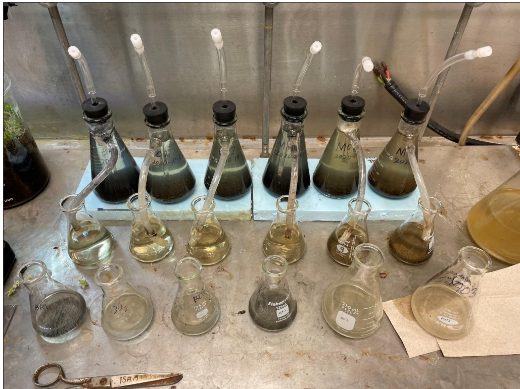
Figure 7. Anaerobic bioleaching flask setup
