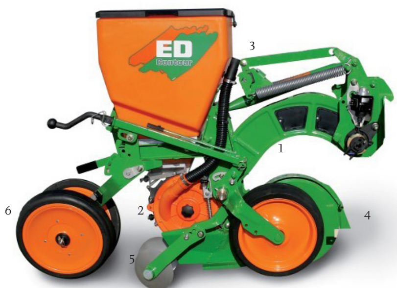
1: The tested seeding unit: 1 - mounting frame; 2 - seed metering unit; 3 - vacuum hose; 4 - disc opener; 5 - closing wheel; 6 - press wheels
