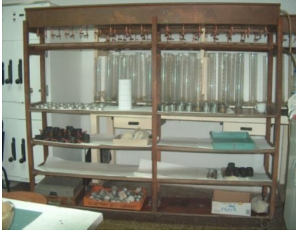
Figure 2. Determination of the filtration coefficient (K-Darcy) in non-disturbed soil samples (in Kopetzky cylinders), on the device designed by Živković
