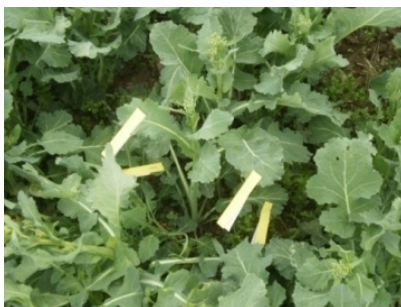
Sl. 4. Biljke uljane repice sa mernim pločicama Fig. 4. Water sensitive papers on oil seed rape plants
