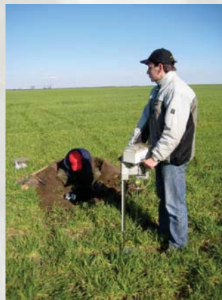
Sl. 1. Merenje otpora konusa Fig. 1. Measuring of cone resistance
