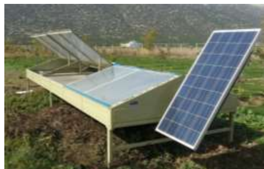
Figure 1 The experimental solar tunnel dryer
