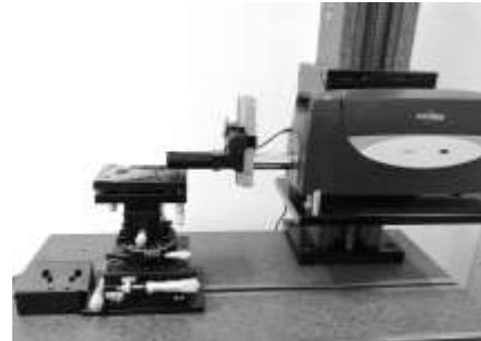
Figure 2 Taylor Hobson rugosimeter used to determine the roughness of the knife blades
