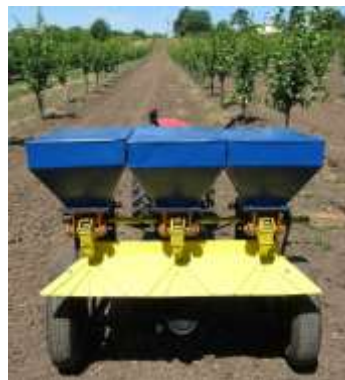
Fig. 4 Granular solid fertilizer delivery equipment:
