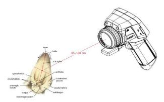
**Figure 1:** Election point (spot) for measuring rabbit ear temperature by infrared camera. Surce of imagines: Anatomy of rabbit ear, ilustration by Gheoghe Constantinescu for Merk, (11) & FLIR® (10).
