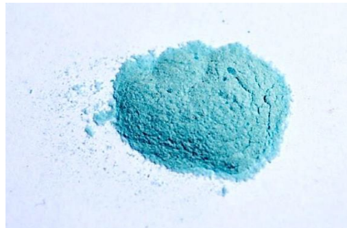
Fig. 2 Macroscopic appearance of the (60-x) \text{B}_2\text{O}_3 \cdot x \text{ZnO} \cdot 34\text{CaO} \cdot 1\text{CuO} with x=5 sample, after being crushed and sieved to <0.075 mm particles
