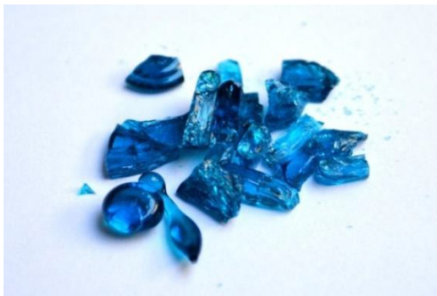
Fig. 1 Macroscopic appearance of the (60-x) \text{B}_2\text{O}_3 \cdot x \text{ZnO} \cdot 34\text{CaO} \cdot 1\text{CuO} with x=10 sample, after being quenched and crushed
