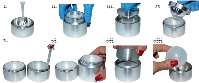
Figure 4-8: Shell fabrication process. i. Mixed and degassed DragonSkin 30 is poured into two hemispherical aluminum cavities of R_o = 25 mm. Only one is shown in i.-iv. , and several layers of tape have been cut into a circle and adhered to the center of one of the hollow spheres. ii. After degassing again, the filled cavity is fitted with an alignment sleeve. iii. A half-sphere of R_i < R_o is inserted. iv. After curing for 25 minutes in the oven, a spherical hemisphere has formed. v. Heptane-diluted polymer is deposited with a syringe to glue two cured hemispheres. vi.-vii. The edges of the two hemispheres are joined and aligned by the alignment sleeve. viii. After curing at room temperature for at least 16 hours, a sealed sphere is removed from the mold.
