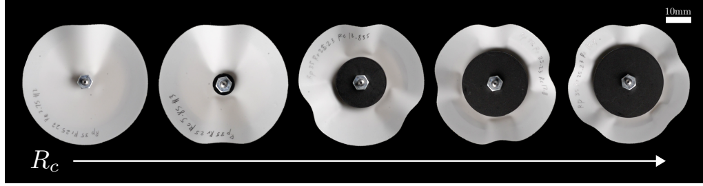
Figure 3-4: Images from experiments at large \epsilon , after the number of cones has reached N_{\max} . R_p and R_r are fixed at 35 mm and 25.23 mm, respectively, and R_c \in \{3.8, 5.9, 13.8, 17.8, 19.7\} mm, increasing from left to right. As the free length R_c increases, so does N_{\max} , from 1 to 5 in these images. In the leftmost image, the clamp is smaller than the hex nut and thus is not visible.
