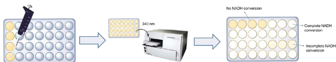
Figure 2.15. Schematic of cryopreservation protocol for monitoring LDH activity. Analysis of freeze/thawed samples either via absorbance spectroscopy. Complete NADH conversion indicated by a complete loss of absorbance.
