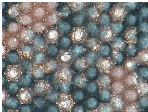
Figure 2. Photograph of the surface of a composite showing the microstructure obtained (CF 4 vol.%, CP 2 vol.%).
