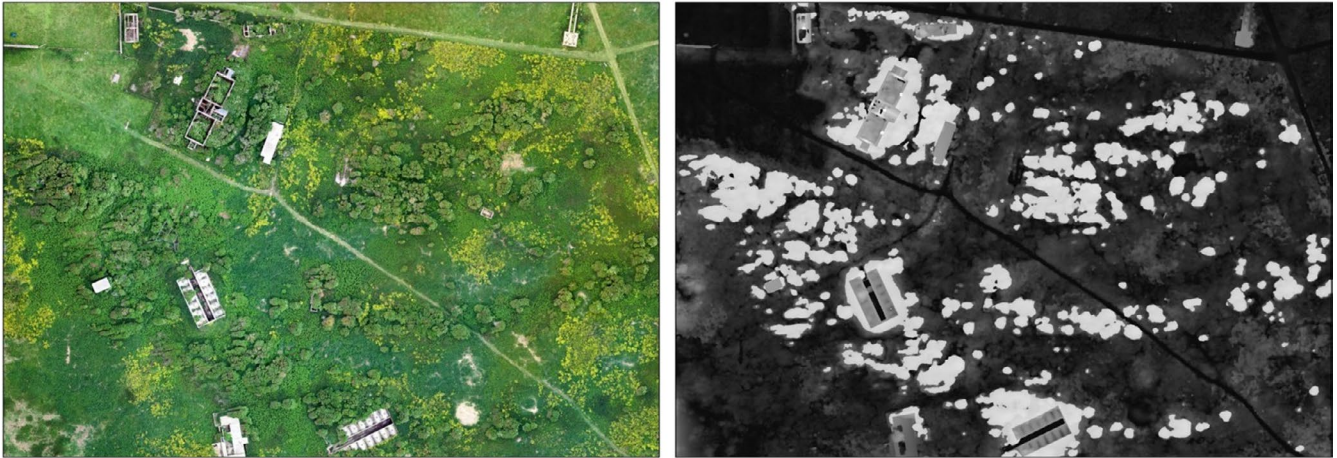
FIGURE 4 Isolation of the scrub layer and buildings on Flat Holm by classifying heights between 1.5 m and 5 m
