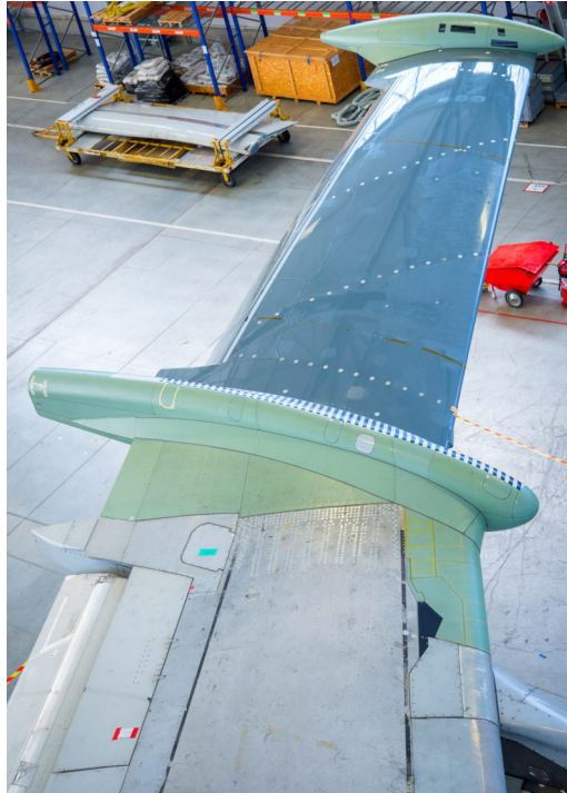
Figure 1.2: Wing extremity of the Airbus A340 used in the BLADE project. The bottom part shows the multitude of natural surface excrescences occurring on a commercial aircraft wing. The mounted NLF wing extension is visible on the upper part and contained step-like and cylinder-like roughness features. © 2017 Airbus. Photograph by P. Pigeyre.
