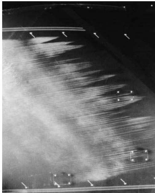
Figure 2.6: Stationary crossflow vortices and transition front on a 45^\circ swept wing visualised with naphthalene at Re = 2.19 \times 10^6 (based on chord) from Dagenhart and Saric (1999)
