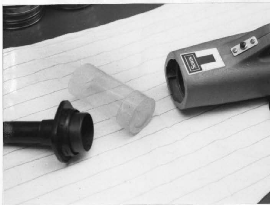
Fig. 3 Break down of portable aspirator. a) Head b) Collection chamber c) Vacuum.
