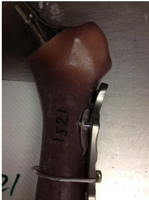
Figure 9: Failure pattern: Unicortical screw pulled out during testing.
