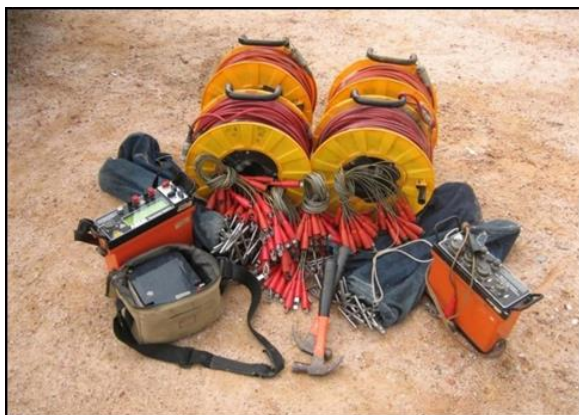
Figure 9: The set of ABEM SAS1000 resistivity meter and ABEM LUND ES464 electrode selector system
