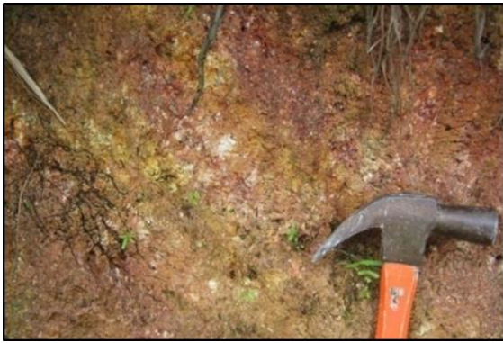
Figure 7: Close-up view of completely weathered granite rock mass shown
