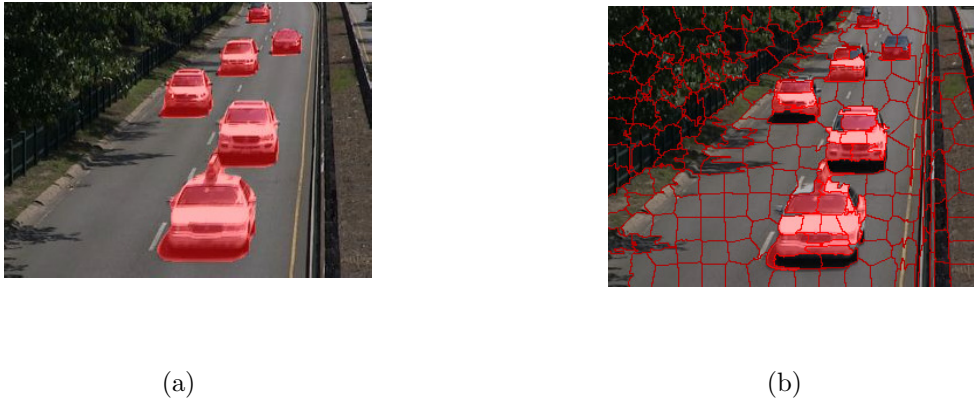
Figure 7.1 Background subtraction implemented on a video frame in (a) pixel-level and (b) SLIC superpixel-level with compactness = 10 and size = 20.
