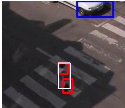
Figure 5.2 Example of the merging of objects. Blue BBs: MOD objects, red BBs: IMOT objects, white BB: resulting fusion of the two inputs into the whole object (pedestrian).
