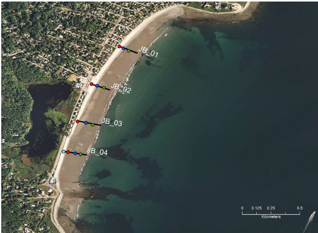
Figure 13. Location map of profile stations and sediment sampling sites during summer, 2015 at Jenness Beach, New Hampshire.
