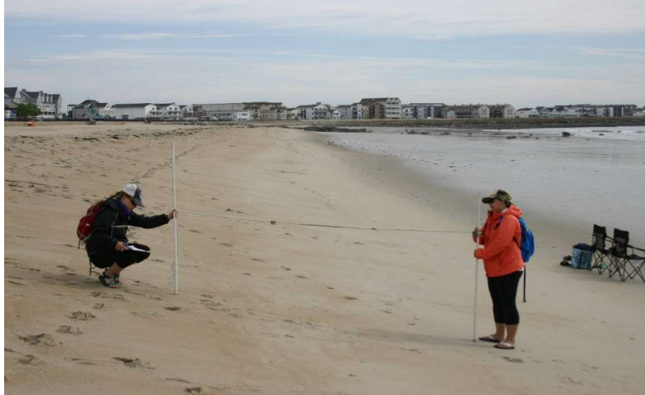
Figure 3. Measuring a beach profile using the Emery method at Hampton Beach on June 18, 2015.
