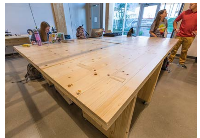
Students and staff in the Fay Jones School used discarded CLT panels from the construction of Adohi Hall to design and build tables for “the cabin” community space (top right and middle right) and for the workshop area (bottom right) of the residence hall. (Photos by Russell Cothren) Students Leopoldo Zepeda (top left) and Corey Booth (middle left) work on the tables during summer 2019. (Photos by Shawnya Meyers)
