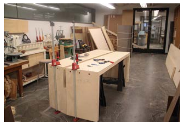
Students and staff in the Fay Jones School used discarded CLT panels from the construction of Adohi Hall to design and build tables for “the cabin” community space (top right and middle right) and for the workshop area (bottom right) of the residence hall. (Photos by Russell Cothren) Students Leopoldo Zepeda (top left) and Corey Booth (middle left) work on the tables during summer 2019. (Photos by Shawnya Meyers)
