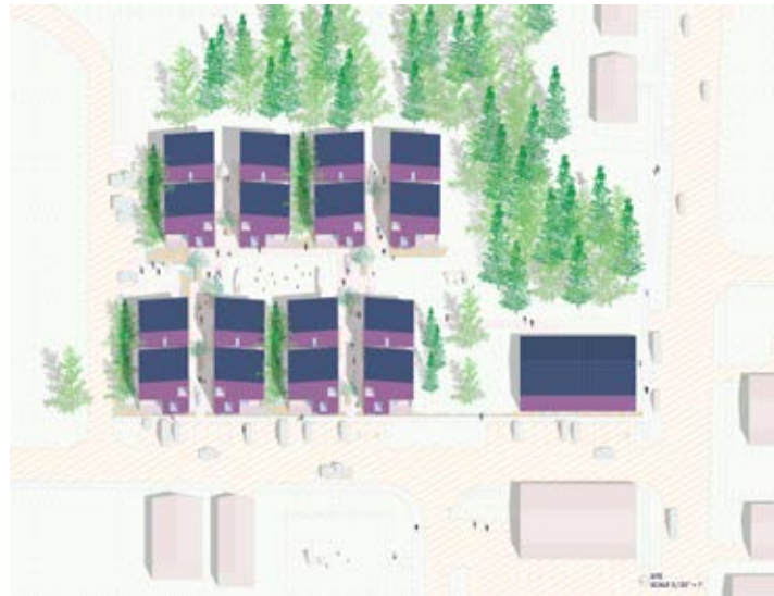
In this site plan for housing for single mothers, three unit apartment buildings are elevated above the flood-prone ground and connected with a boardwalk and communal play spaces. Drawn by Tamsan Mora and Ashley Navarrete.
