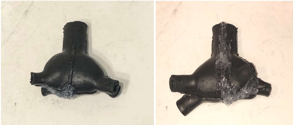
Figure 5. Conductive silicone atrium.
