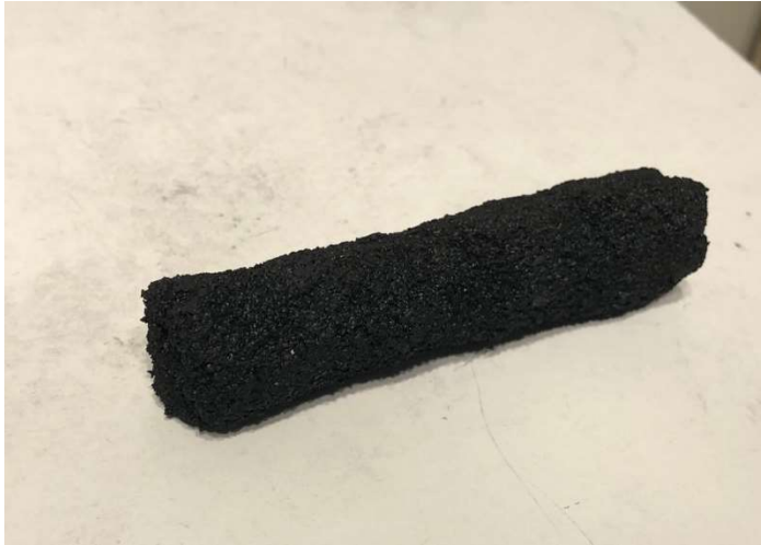
Figure A1. Cylindrical conductive silicone sample for resistivity measurement
