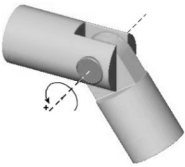
Fig. 30. Revolute joint: one degree of freedom.
