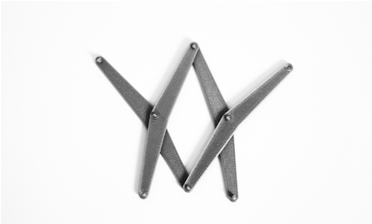
Fig. 21. Angulated scissors mechanism capable of two-dimensional expansion.
