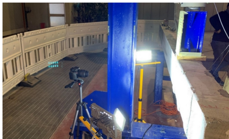
Figure 2. Digital Image Correlation (DIC) system adopted for strain monitoring.
