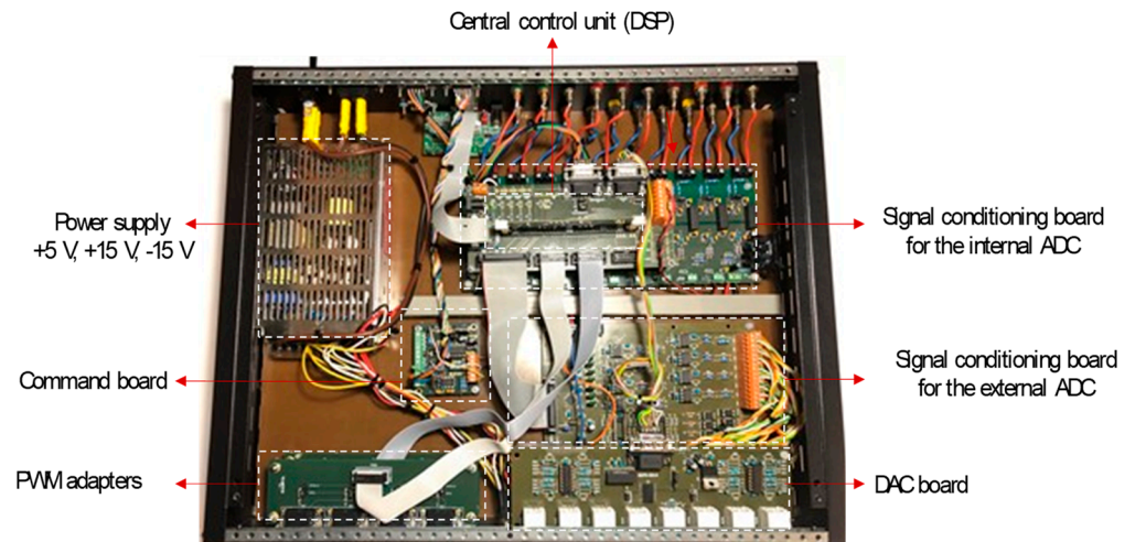
Figure 14. Control system hardware fitted in a metallic box.
