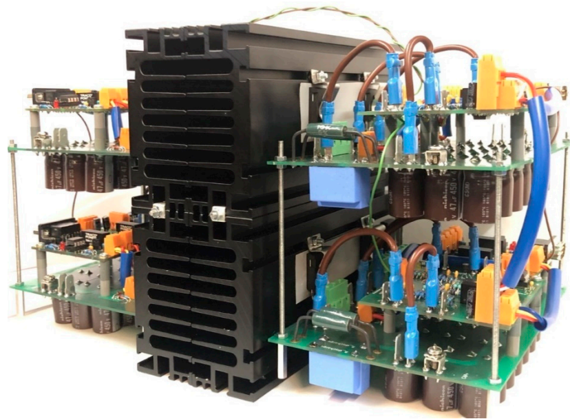
Figure 12. Single MMC leg/phase (four submodules).
