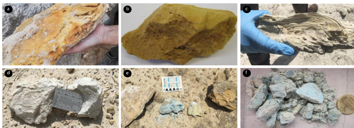
Figure 4 Typical hardpan. a) Banded Fe-rich hardpan cemented by jarosite and goethite; b) Fe-rich hardpan mainly composed by massive jarosite; c) and d) fragile hardpans, mainly cemented by kaolinite; e) and f) Light blue As-rich hardpans
