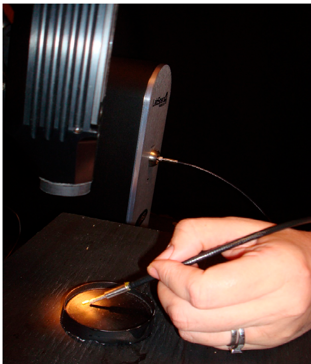
Figure 2. Demonstration of measuring reflectance from an insect with the Analytical Spectral Devices (ASD) Labspec 4 Spectrometer.
