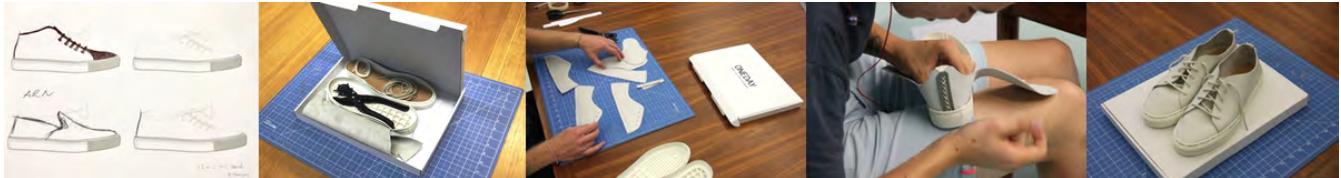
Figure 1. The ONEDAY Toolkit being used to make a pair of personalized shoes.
