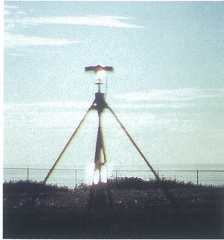
Fig. 3. GPS site installation. Wyatt-style drilled braced monument installed at Cape Blanco, Oregon. Each of five pipes drilled to approximately 12 meters depth, set in non-shrink grout and isolated from soil and ground motions in the upper 4 meters by padded casing. The Pacific Northwest offers challenging conditions for stable site conditions. Much of the area is underlain by pervasively jointed volcanic rocks, poorly consolidated Tertiary strata, or other unstable lithologies. This monument was designed to provide stability under such conditions.
