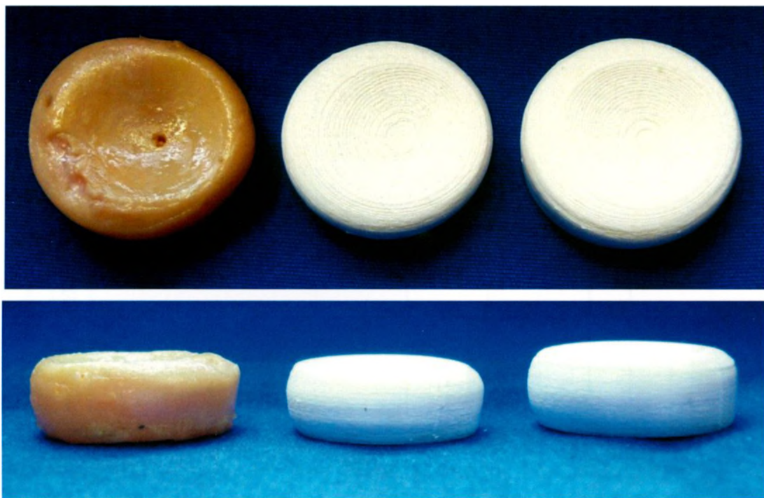
Figure 4.9: Comparison of native anatomy (left) to patient-specific (middle) and quasi-anatomic (right) implant designs, before sanding and coating of the implant surface.
