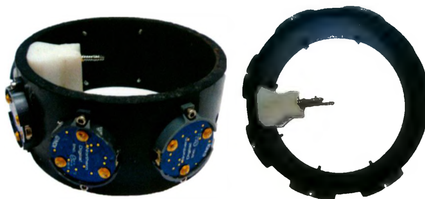
Figure 4.5: The “ring” used to track the position of the radius.
