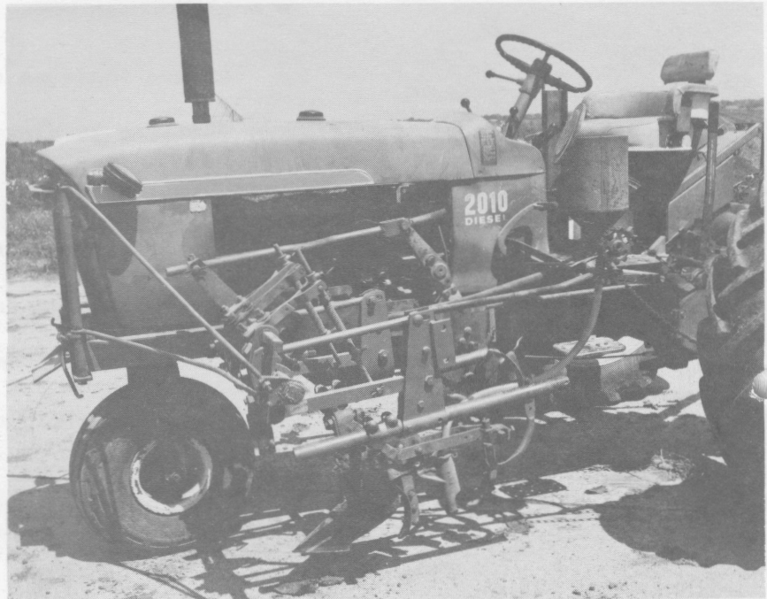
Figure 3. Tractor-mounted modified Planet Junior used to plant honey mesquite and huisache seed.
