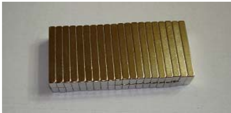
Fig. 37 NdFeB permanent magnets.
