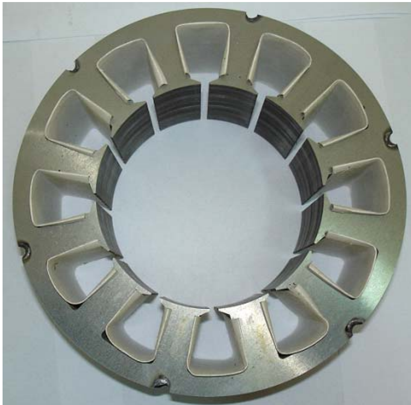
Fig. 33 Stacked lamination stator core.
