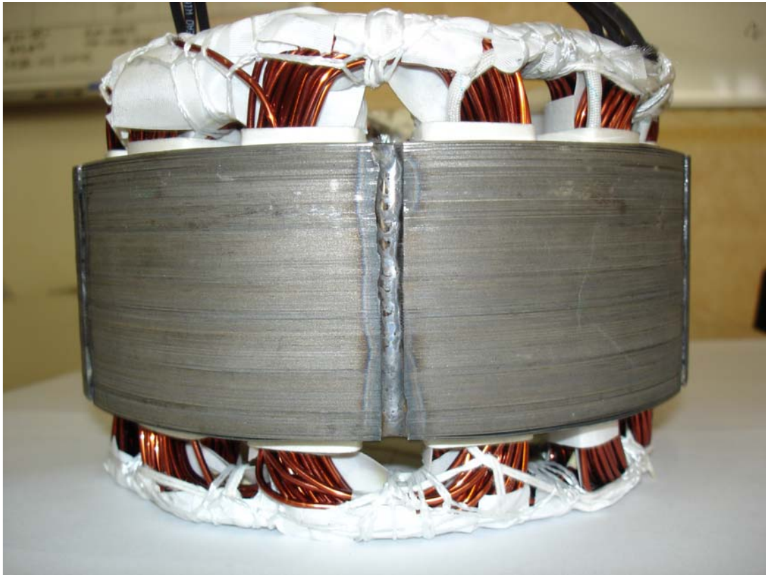
Fig. 34 Side-view of the stator winding configuration.
