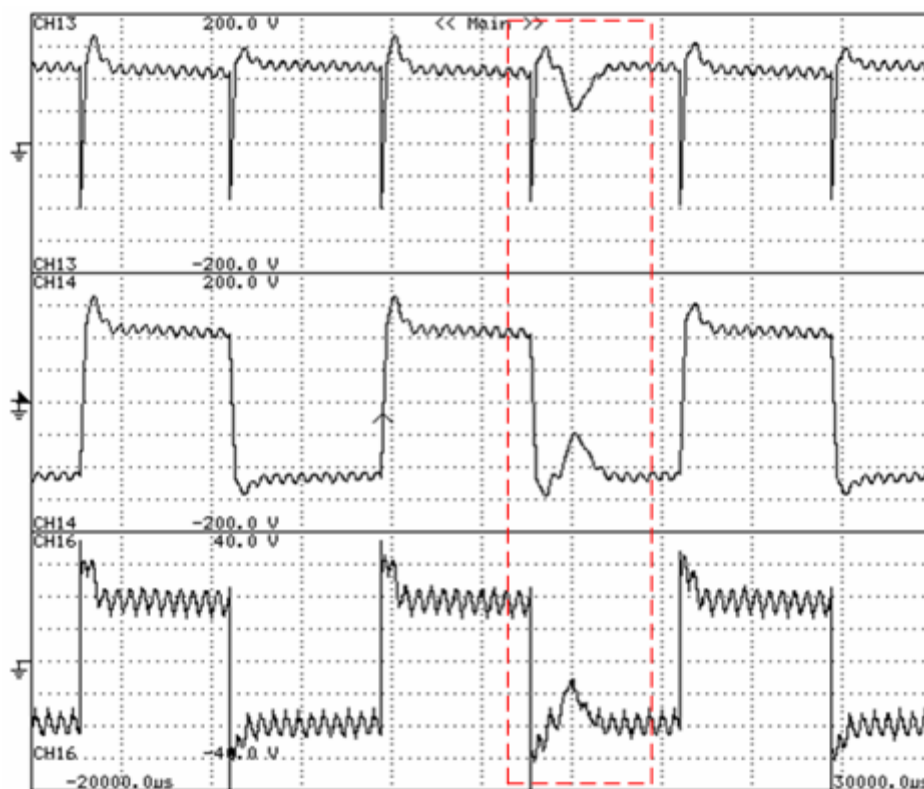
Fig. 72 Experimental waveforms of single-phase output at transient condition. From top to bottom : (a) DC link voltage (50V/div) (b) single-phase output voltage (50V/div) (c) single-phase output current (10A/div)
