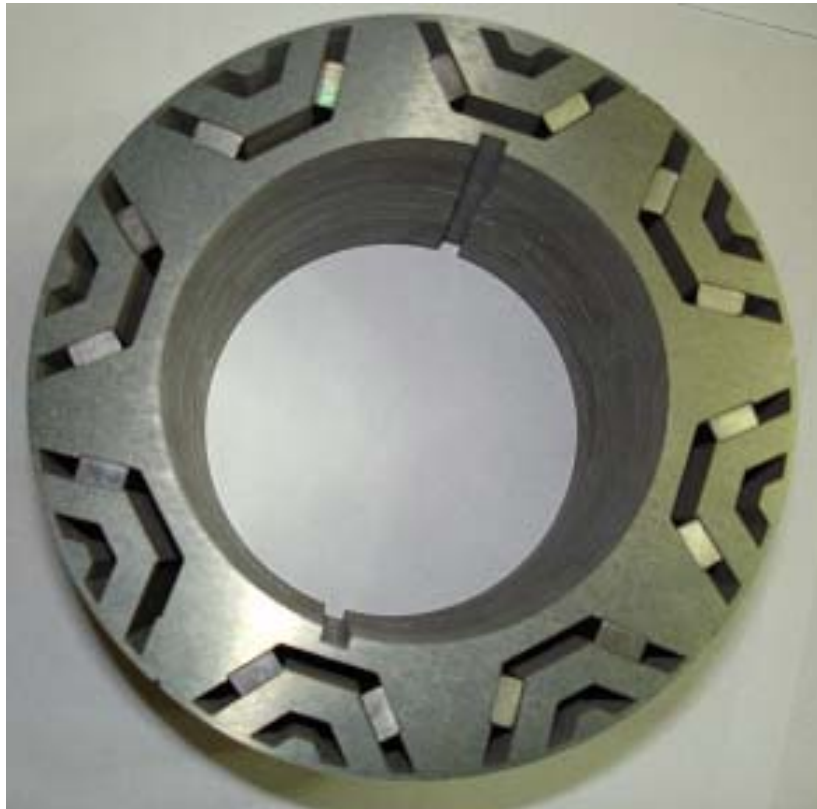
Fig. 38 Stacked lamination rotor core and inserted PMs.
