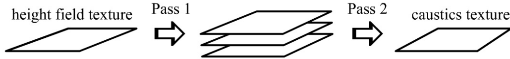
Figure 5.12. The two-pass algorithm: the first pass reads the height field texture and generates multiple outputs; the second pass reads the result of the first pass and produces the final caustics map.
