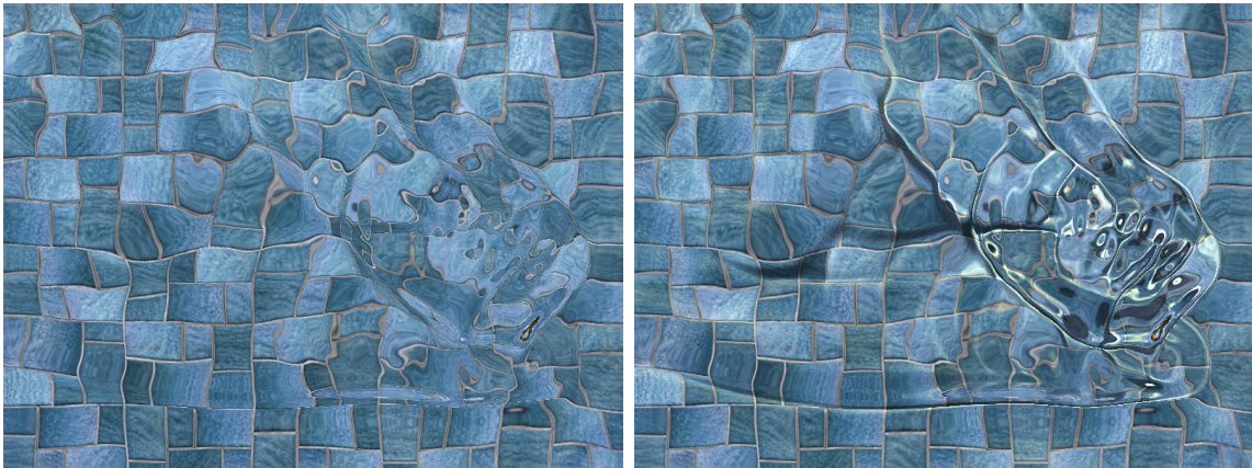
Figure 5.9. A height field water surface rendering with and without caustics. The image on the left only has reflections and refractions. The image on the right shows the same water surface with caustics computed using our fast caustics computation method for height field surfaces.
