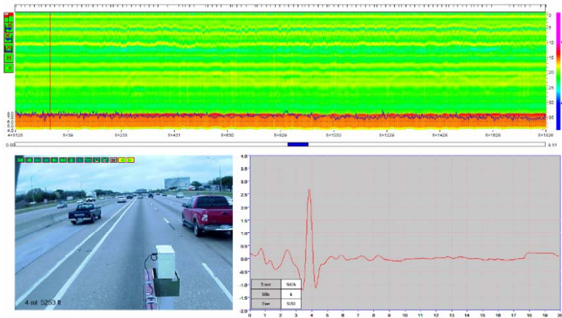
Figure 3-32 GPR Image of Sampled Section on IH 635.
