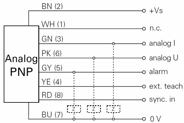
Fig. 3.19. Laser sensor connection diagram [25].
