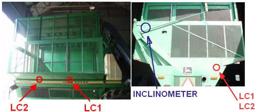
Figure 4. Mounting locations of sensors
