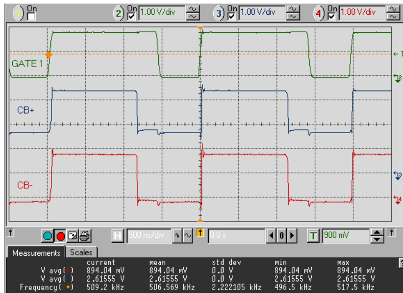
Fig. 127. Measured waveforms across bootstrapped capacitor C_3
