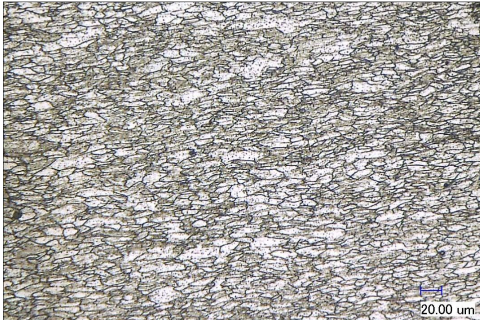
Fig. 82. Optical micrograph of ECAE: IF steel sheet (route 2A) on the longitudinal plane.
