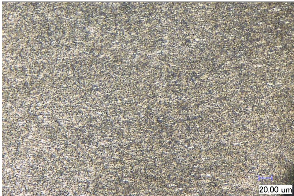
Fig. 84. Optical micrograph of ECAE: IF steel sheet (route 4A) on the longitudinal plane.
