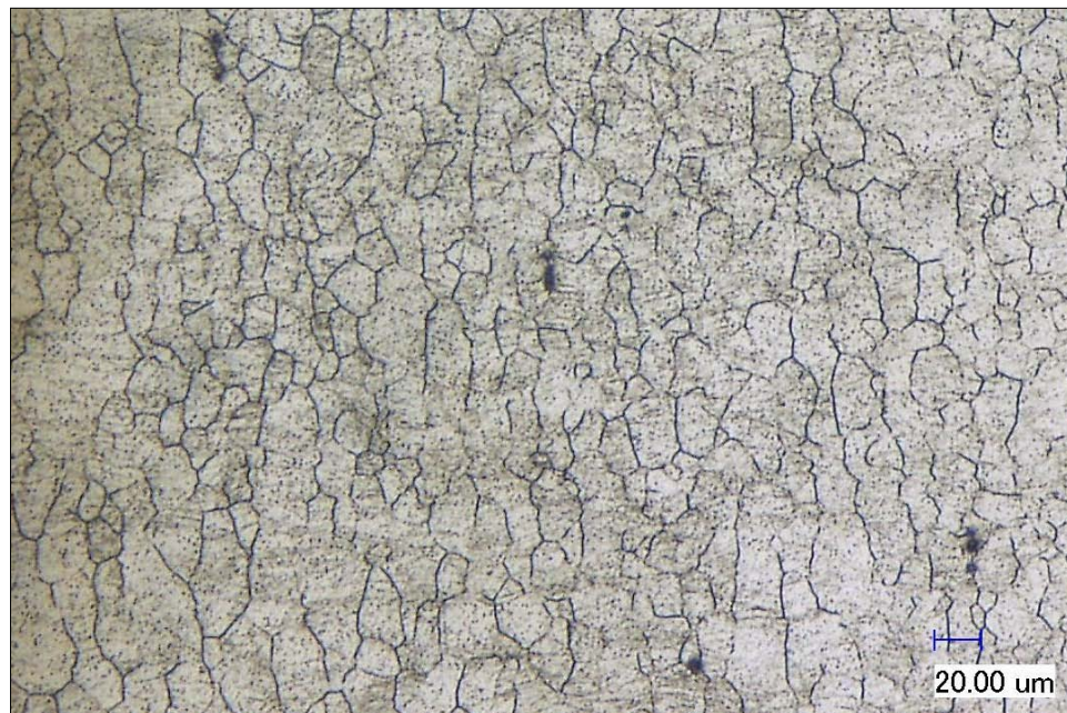
Fig. 85. Optical micrograph of ECAE: IF steel sheet (route 4C) on the longitudinal plane.
