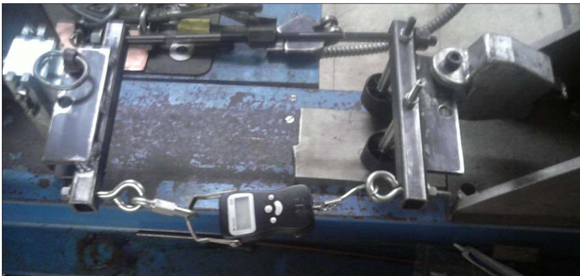
Fig. 60. Schematic of assembly used for drawing force measurement.
