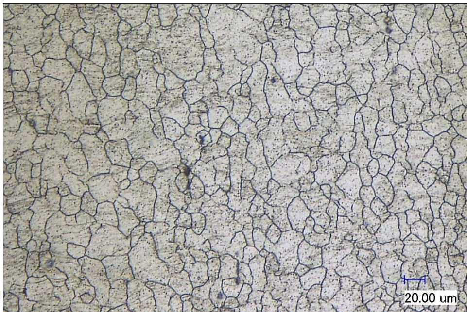
Fig. 83. Optical micrograph of ECAE: IF steel sheet (route 2C) on the longitudinal plane.
