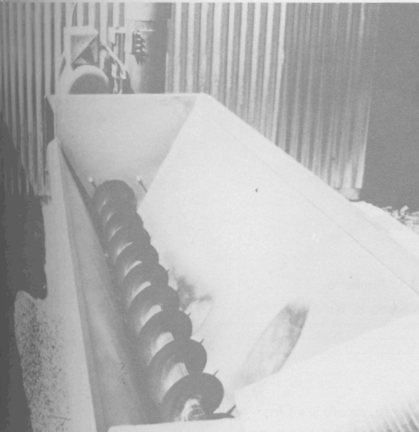
Figure 5. A vertical auger with feeding hopper for elevating grain from trucks to storage bins.
