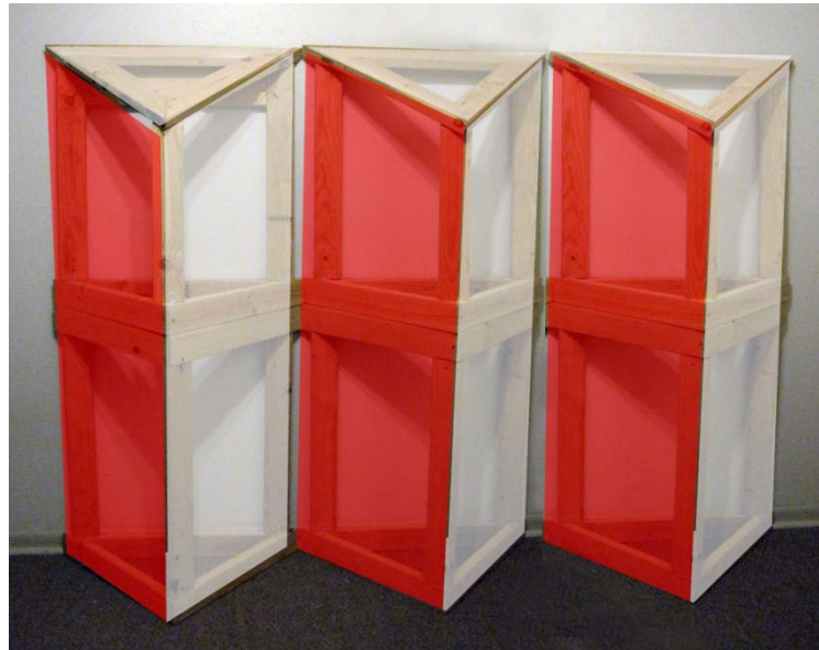
Fig. 28. Supporting frame showing modularity
