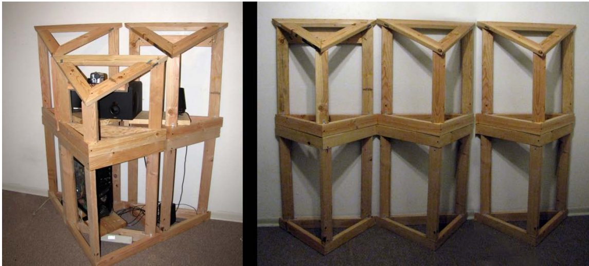
Fig. 27. Constructed supporting frame showing modularity
