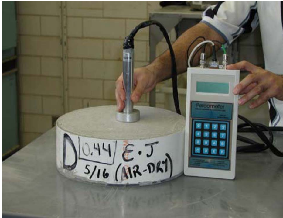
Figure 4-19 Measurement of composite dielectric constant of concrete sample (Avelar Lezama 2005)
