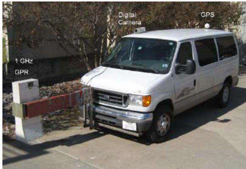
Figure 2-15 TTI's GPR vehicle with digital camera and GPS (Liu and Scullion 2009)
