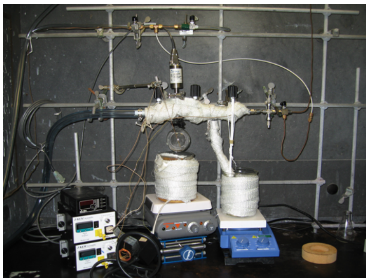
Figure 3.2. Photograph of the homemade CO oxidation reactor system. The pressure of the reactor flask was measured by a Baratron Pressure Transducer and the temperature of the oil bath and manifold were controlled by J-KEM Scientific temperature controllers.
