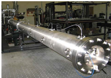
Figure 17. Shock-tube facility at Texas A&M Turbomachinery Laboratory, design and construction by C.J. Aul and J. de Vries
