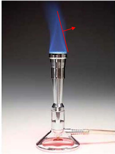
Figure 24. Bunsen flame, flame speed equal to v_u \sin \alpha
