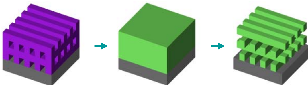
Figure 31. The process of fabricating 3D inorganic structure with 3D polymer template.
