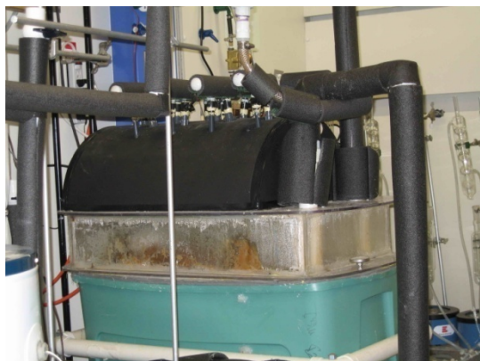
(c) Biomass treatment "bed" to hold bagasse.
