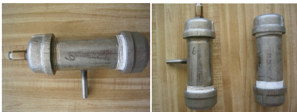
Figure 4-8. Self-constructed high-pressure reactor for rapid batch ammonia pretreatment (24 hours).
