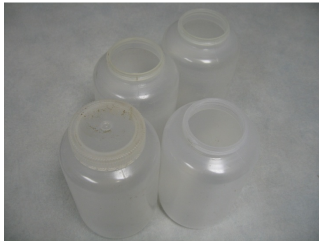
Figure 4-10. Beckman 1-L centrifuge bottles (Nalgene brand NNI 3120-1010) for batch ammonia pretreatment.
