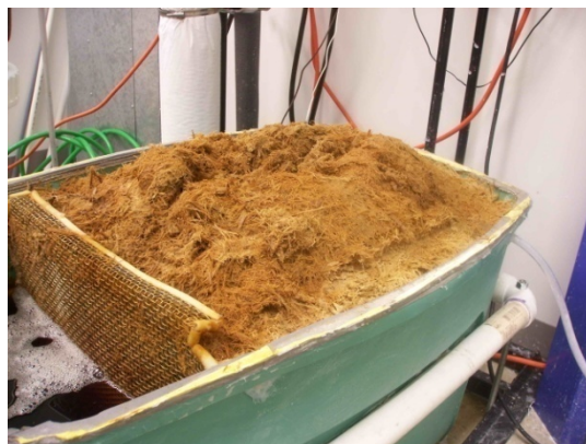
(d) Harvested bagasse after air-lime treatment with a treatment time of 2 months.
