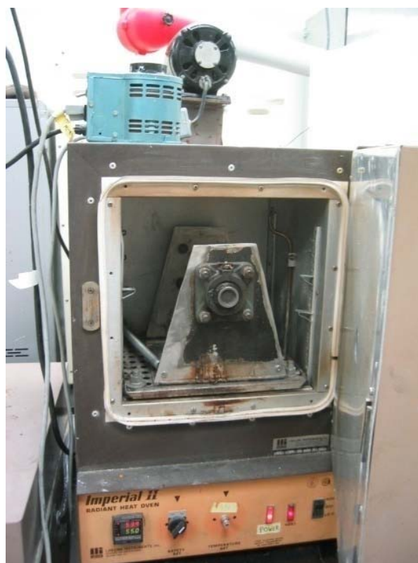
Figure 4-7. Modified temperature-adjustable oven for rapid batch ammonia pretreatment (24 hours).
