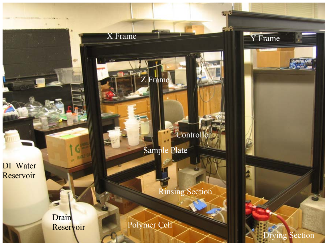
Figure 21. Image of robotic dipper built for LbL assembly.
